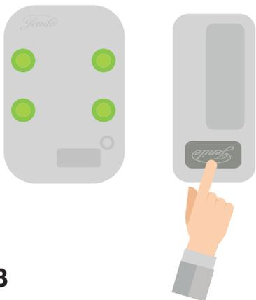
3. Immediately actuate the transmitter after having pressed the plug (ring the bell, press on the remote control, shout in the baby crying detector, ...)
