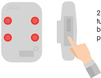
2. Press the plug button (C) until the vibrator turns red (WARNING: do not hold down the button too long, you are at risk of deleting all previous connections)
