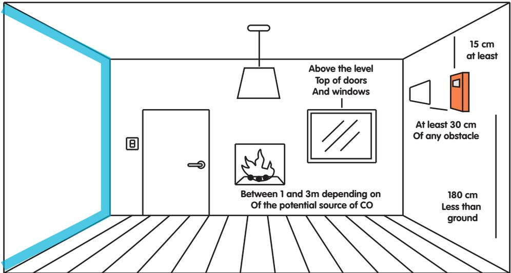
In the room where the combustion appliance is located: The detector must be placed Between 1 and 3 m horizontally from the potential source of CO, to at least 1.80 of the soil And 15cm from the ceiling. In the rooms to be lived: relatively close to the space where Breathe the occupants
